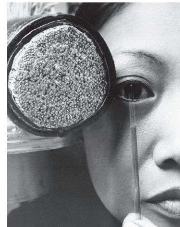
FIGURE 1.10 The small cable on the right contains 144 glass fibers and can carry more than three times as many telephone conversations as the traditional (and much larger) copper-wire cable on the left. (© Bettmann/CORBIS.)
