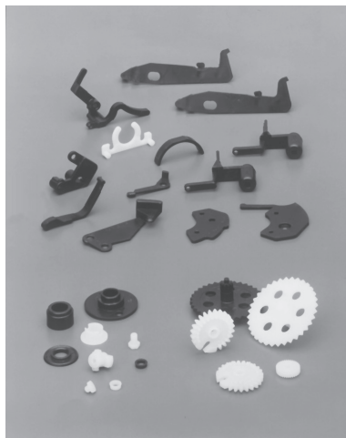
FIGURE 1.11 Miscellaneous internal parts of a parking meter are made of an acetal polymer. Engineered polymers are typically inexpensive and are characterized by ease of formation and adequate structural properties. (Courtesy of the DuPont Company, Engineering Polymers Division.)
